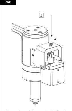
Ensure air supply is connected to the pin close supply.
