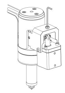
Ensure the closing air supply is on. Use a hex key in the pin stop screw to adjust the pin to the correct position.
