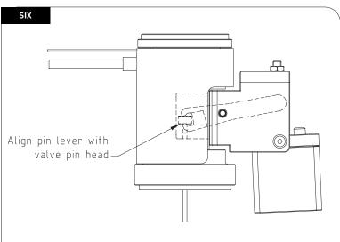
Fit cylinder assembly to cylinder bracket taking care to align pin lever with valve pin head, and fit lever pivot pin and cylinder pivot screws.
