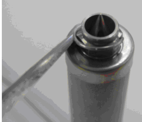
Figure 58: Remove an X Range Snap Ring
