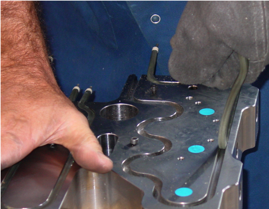
Figure 49: Pull Pressed-in Heaters out of Straight Sections
