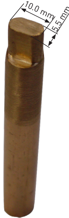
Figure 52: Using a Soft Brass Tool to Finish Heater Installation and Close Up of Tool
