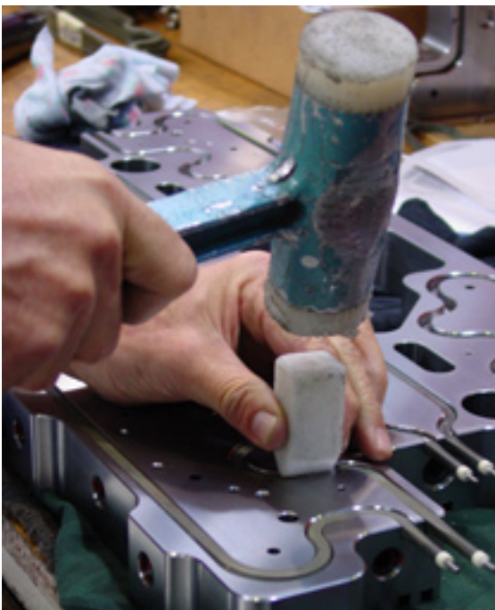
Figure 51: Using a Plastic Wedge to Hammer the Heater onto the Bottom of the Heater Slot
