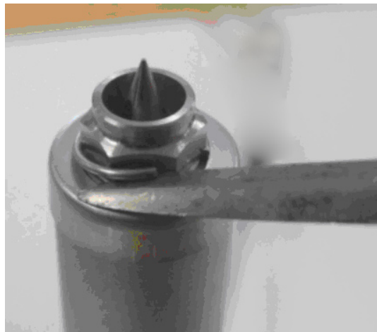
Figure 57: Wedge a blade under a X Range Nozzle Snap Ring
