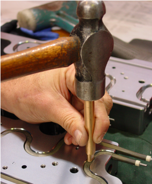
Figure 52: Using a Soft Brass Tool to Finish Heater Installation and Close Up of Tool
