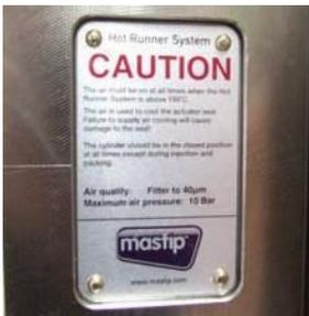
Fit the name plates and caution plates using the hammer drive rivets.
