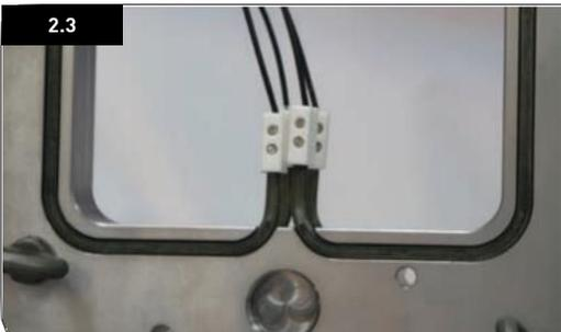
**Fit ceramic terminals to manifold heater**
