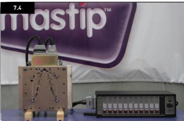
**Connect controller unit & confirm wiring order is correct.**
