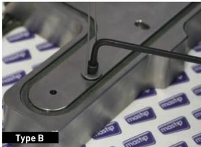
**Fit thermocouples to manifold**
