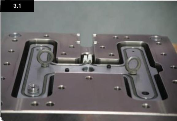
**Lower the manifold into the pocket**
