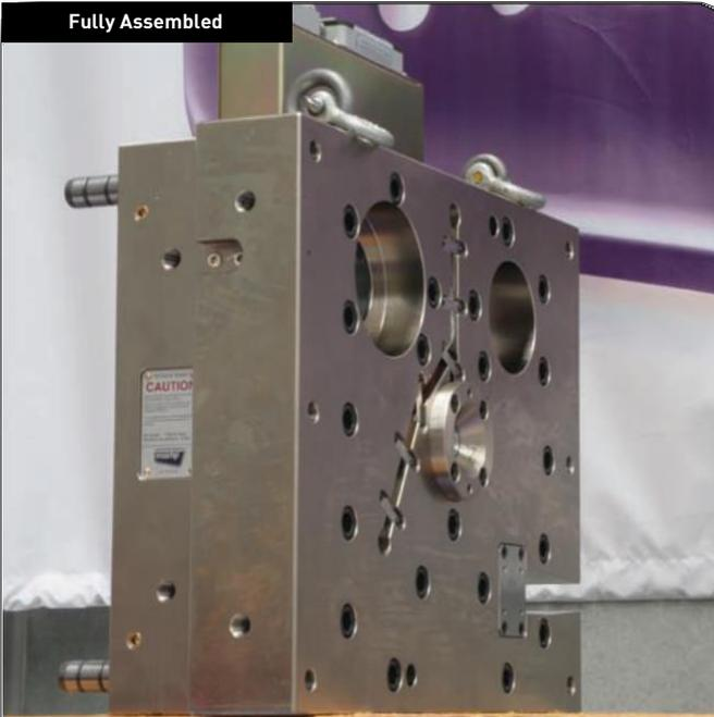
Fully assembled hot half from sprue side.
