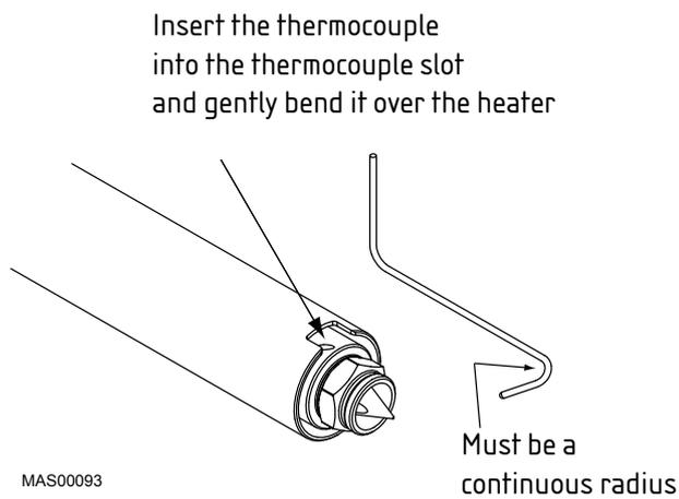
Figure 27: Install Thermocouple on MX Nozzle
