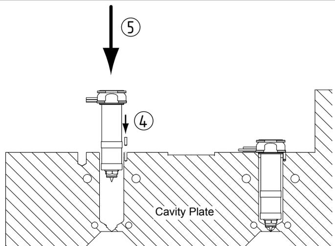
Figure 37: Insert Dowel and MX Nozzle
