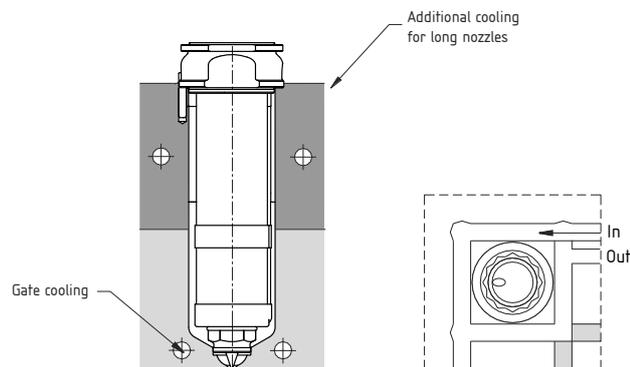
Figure 13: Cooling Channels Example
