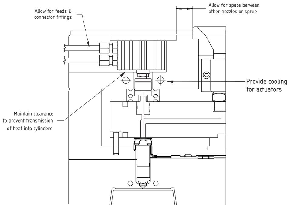
Figure 11: Mould Modifications for Valve Gate Applications
