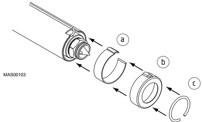
Figure 36: Finish MX Nozzle Installation
