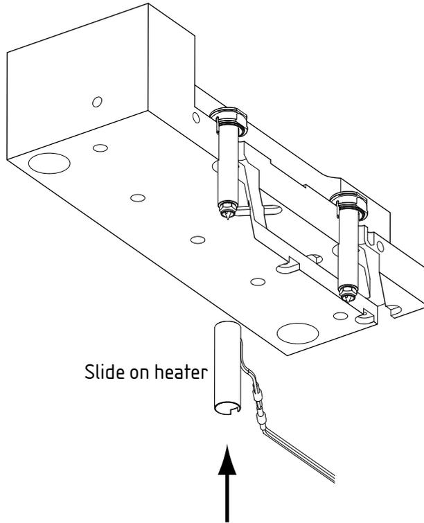
Figure 30: Slide on MX Heaters
