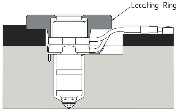
Step 6: Fit the Locating Ring and tighten retaining screws.
