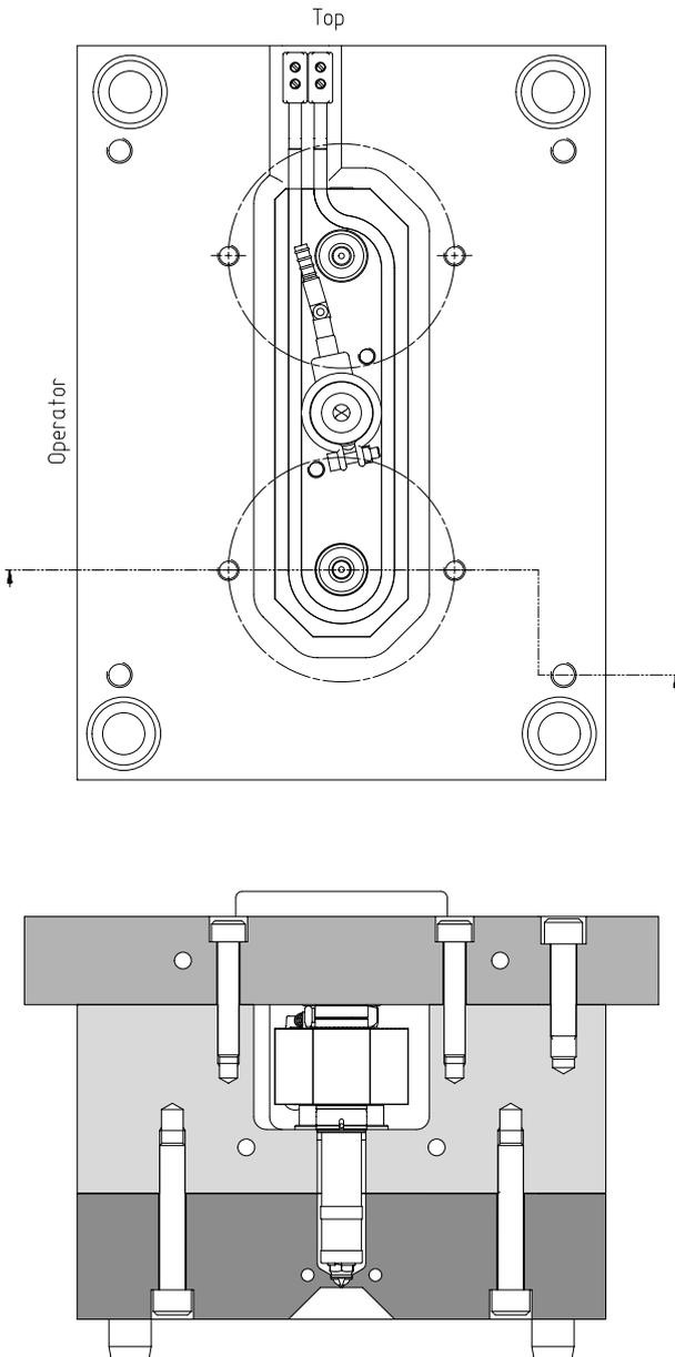
**Figure 12: Suggested Placement of Clamping Bolts**
