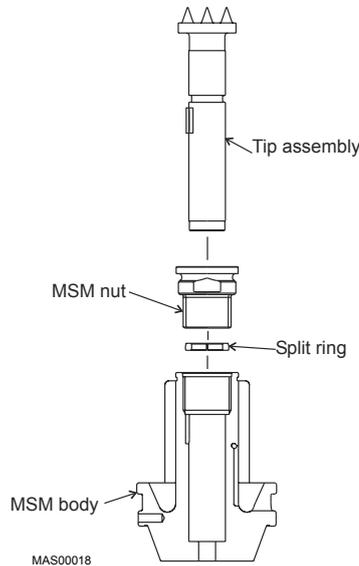
**Figure 91: Reassemble MSM Nozzle**
