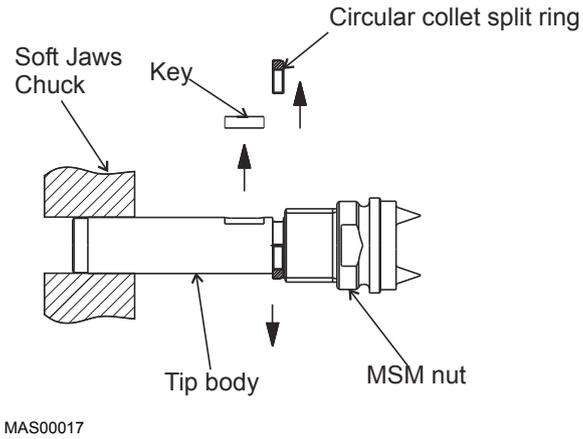
**Figure 90: Remove MSM Key and Collet Halves**
