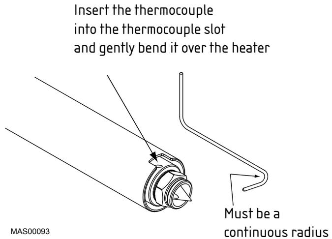
Figure 80: Replace BX or SX Thermocouple
