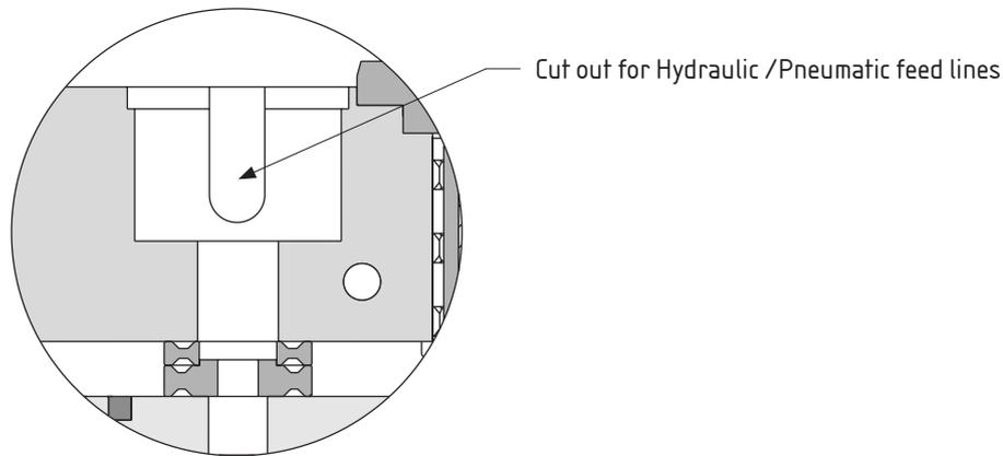
**Figure 2: Slots for Feed Lines**
