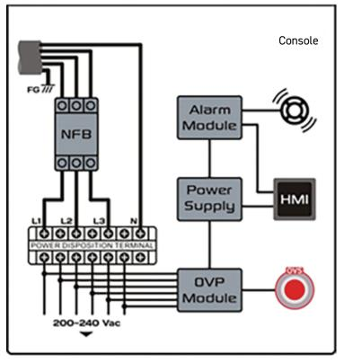
Control Cabinet Wiring Diagram
